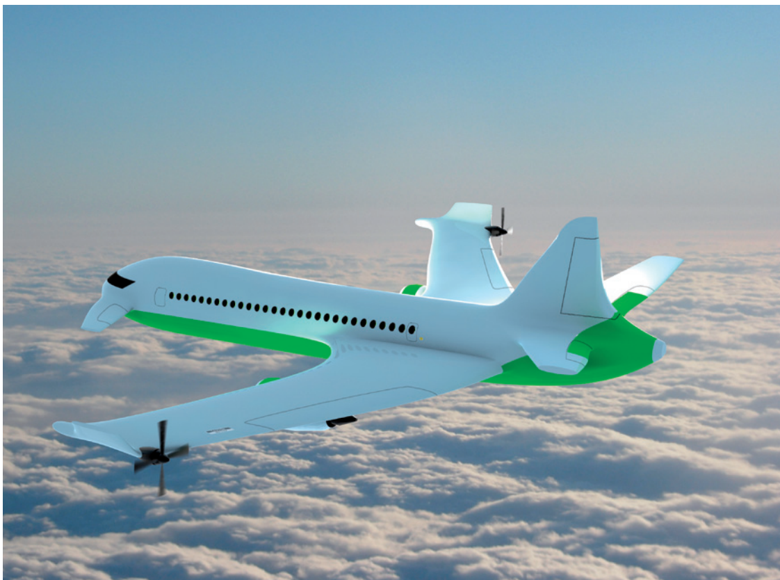
◀ Fig.32. Artist's impression of wing mounted generators to retrieve energy from the vortex produced when flying
